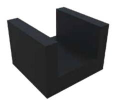
Rubber Joist Isolation Clips are used as a highly effective way to isolate and decouple floor joists from the subflooring. By decoupling the floor joists, the room is able to be isolated from its surrounding structure. Rubber floor joist isolators simply snap onto any "2x" joist or stud (2x4, 2x6, etc) and do not require any fastener that could harm the isolation value.
